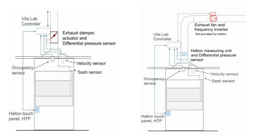
Figure: Double Sensor Control with centralised and single exhaust fan ventilation
