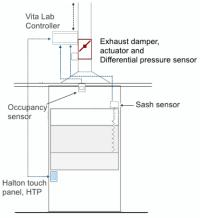
Zone solutions for total room control and enhanced duct pressure control .
