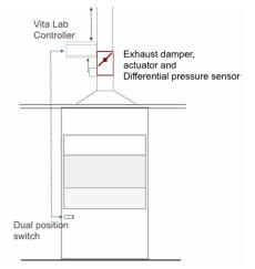
Figure: Dual Position Control, centralised exhaust ventilation
