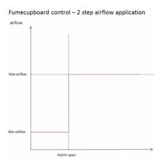
Figure: Dual position airflow control
