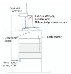
Figure: Sash Position Control, centralised exhaust ventilation
