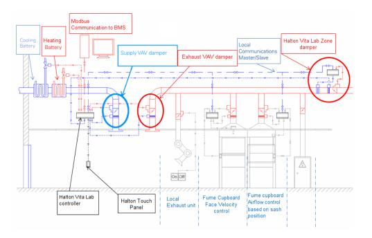
Fig. Total Exhaust Measurement with Supply and Exhaust control and temperature control
