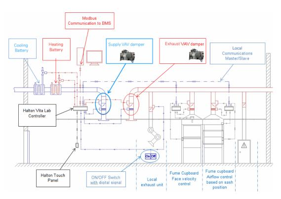
Figure: Room Airflow Control - Supply and Exhaust Control configuration
