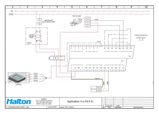
Figure: Supply Airflow Control wiring diagram
