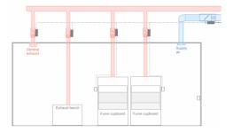
Fig: Centralised exhaust
