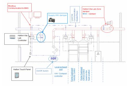
Figure: Room Airflow Control with Supply Control configuration
