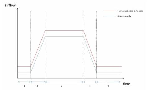
Figure: Room airflow control
