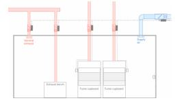
Figure: Single exhaust fan ventilation
