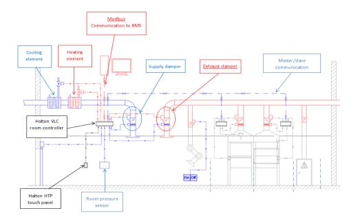
In the communication between the system components, local communication is used. The Halton Vita Lab Room Controller (VLC/RC) is mounted on the master damper (supply in case of underpressure mode, and exhaust in case of overpressure mode). The VLC/RC functions as the master controller and the fume cupboard controllers (VLC/FC) as slaves. The Halton Vita Lab room master controller coordinates the communication as follows
